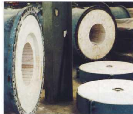
10: Lined reactor components
